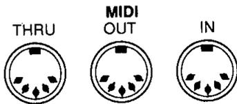
**IN:** The terminal by which this instrument receives data from other equipment.
